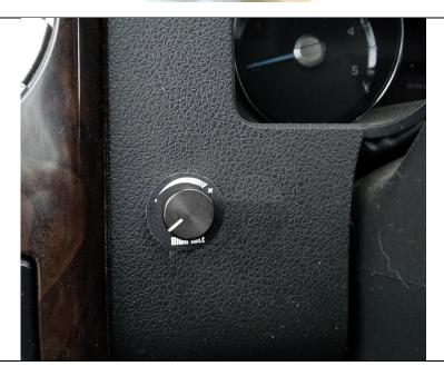
If mounting in the knee bolster, be aware of the reinforcement plate behind the bolster which will limit the available spaces to mount the switch.
