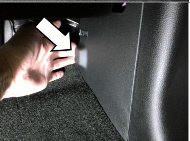
Locate and disconnect the OEM up-fitter wire pigtail. This pigtail will not be used so it may be left in the glove box or tucked back in the fuse box area.
