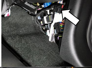
Plug in the BD High Idle wiring harness to this connector.
