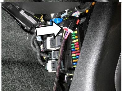
Tuck the wire from the BD High Idle kit behind the carpet/under the dash towards the driver side of the cab. You can remove the lower center console trim to make this easier. Wire may be secured with supplied zip ties.
